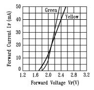
Fig.2 Forward Current vs. Forward Voltage
