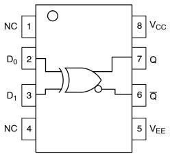
Figure 1. Logic Diagram and Pinout Assignment
